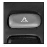
The hazard warning button is located on the instrument panel near the comfort controls.
